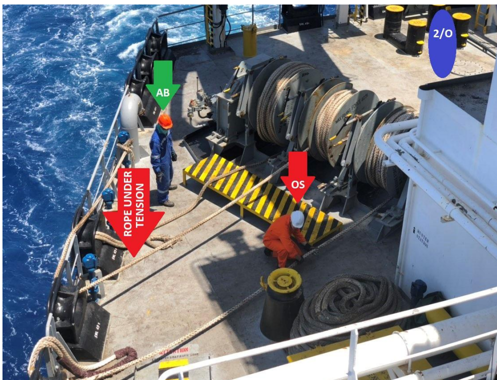
Figure 4.3/2: The actual arrangement of the stbd stern and the positions of the 2 nd Officer, the A/B near the stbd winch controller and the O/S who at the time of the casualty was stowing the fore mooring rope on its drum, with his back turned to the mid mooring line, which was under tension.
