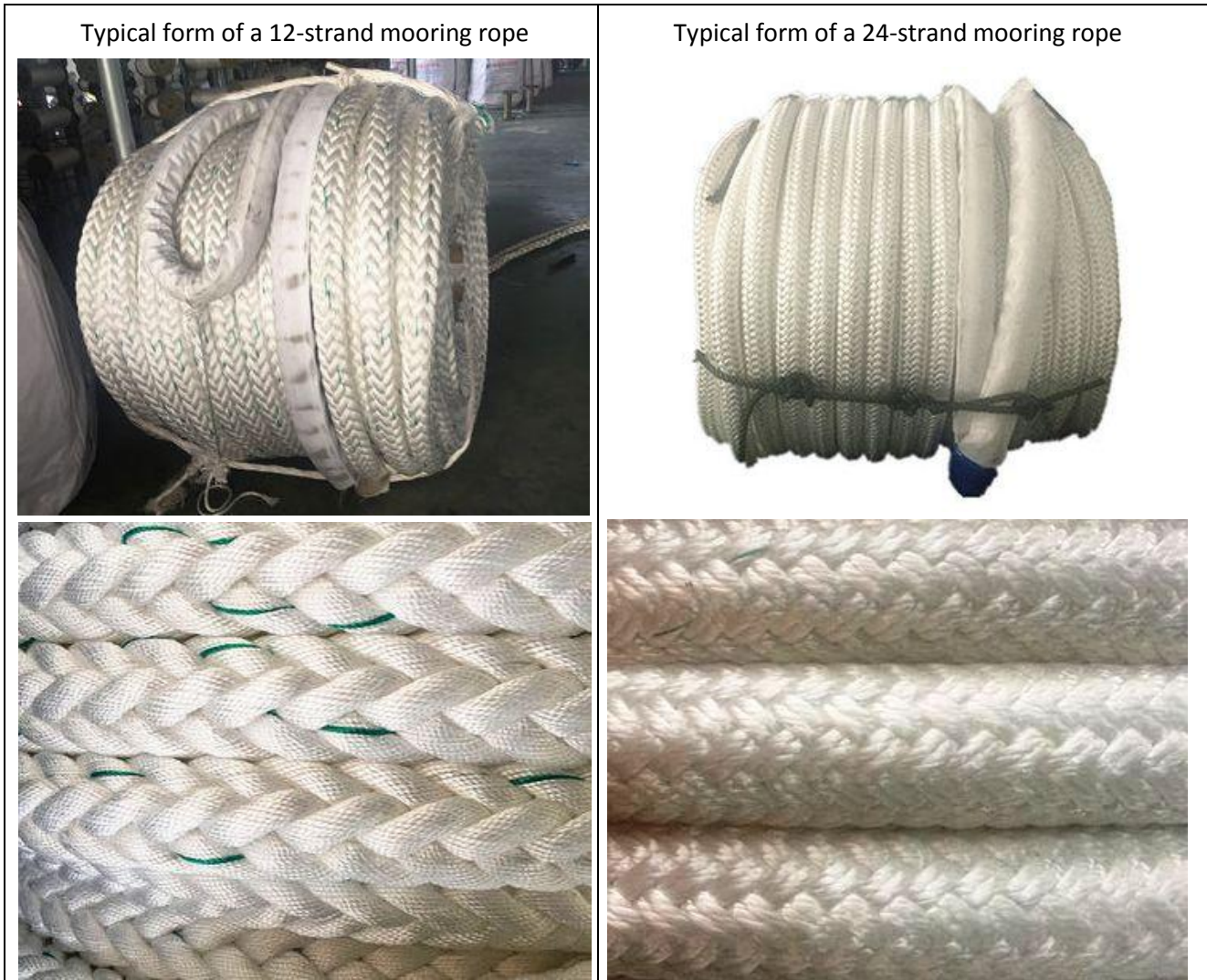
Figures 4.2.2.4 / 3, 4, 5 & 6: Comparison of the form of a 12-strand rope (left side) and a 24-strand rope (right side).
