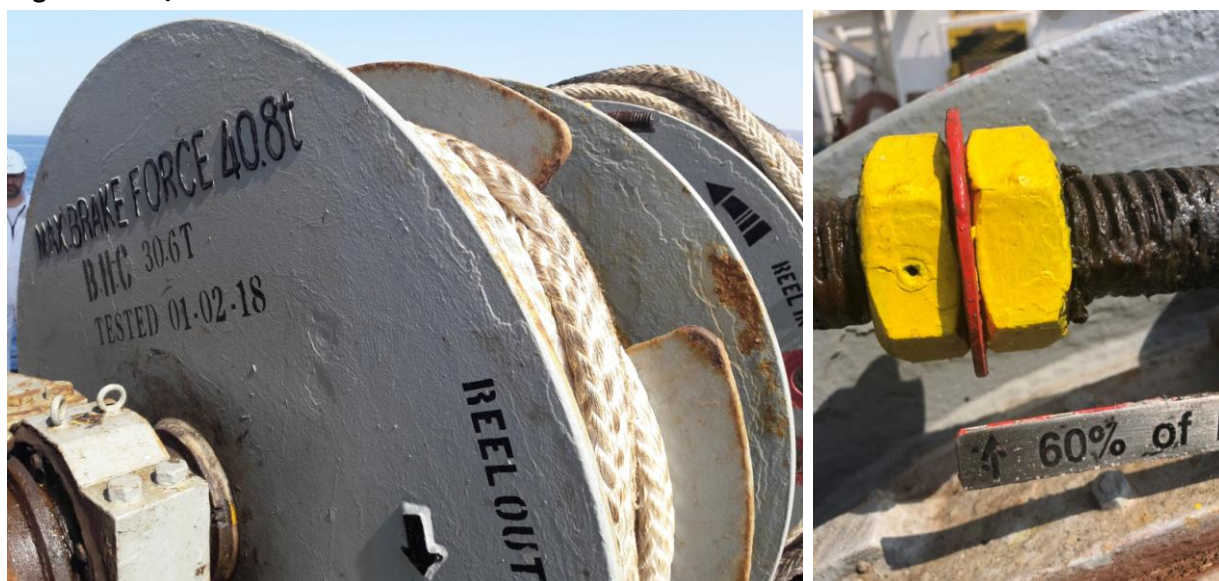
Figures 4.2.1/2 & 3: The signings written and fitted on the drum and on the brake tightening screw following the last brake test of 1 st February 2018.
