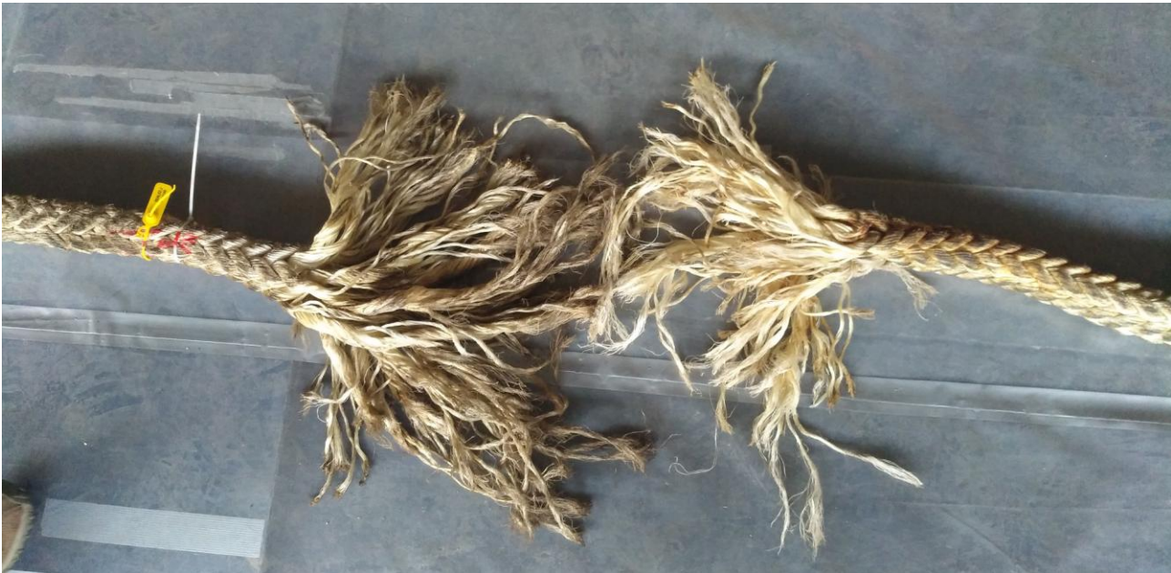
Figure 4.2.2.1/1: The rope's breaking point at the part that remained onboard (left part of the photo) and at the part that remained on the terminal's bollard (right part of the photo).
